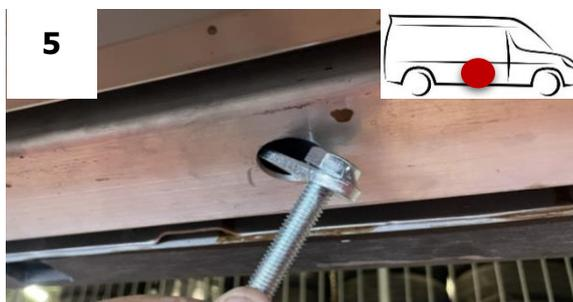
Insert HTC OR8 into the hole and fasten the M10x50 rod.
