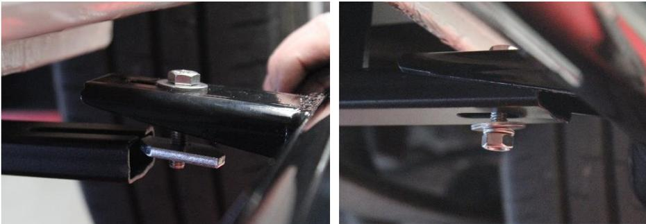
**Important!** After positioning the step in the appropriate position, tighten the M8 nuts with 25 Nm and the M10 nuts with 50 Nm.
