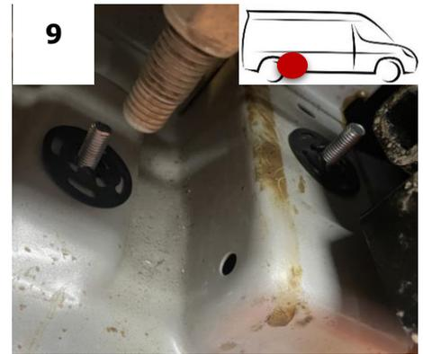
Rear bracket to the vehicle with the help of M10 nut.
