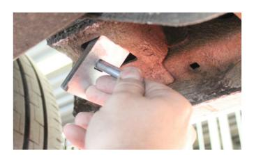
Place the right bracket on the Bolt and tighten with nut (NR 15)
